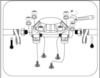
Fix the G3/4 connectors to inlets of the body. Push the body over floor screws and fasten with steel gasket and nut. Connect the body with hot (Left) and cold (right)water pipes using thread seal tape.
