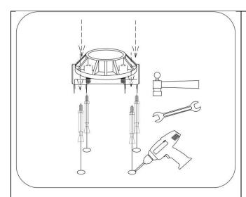
Mark out the fixing positions on the flooring basing on the body and drill four holes. Fix the floor screws into the holes.
